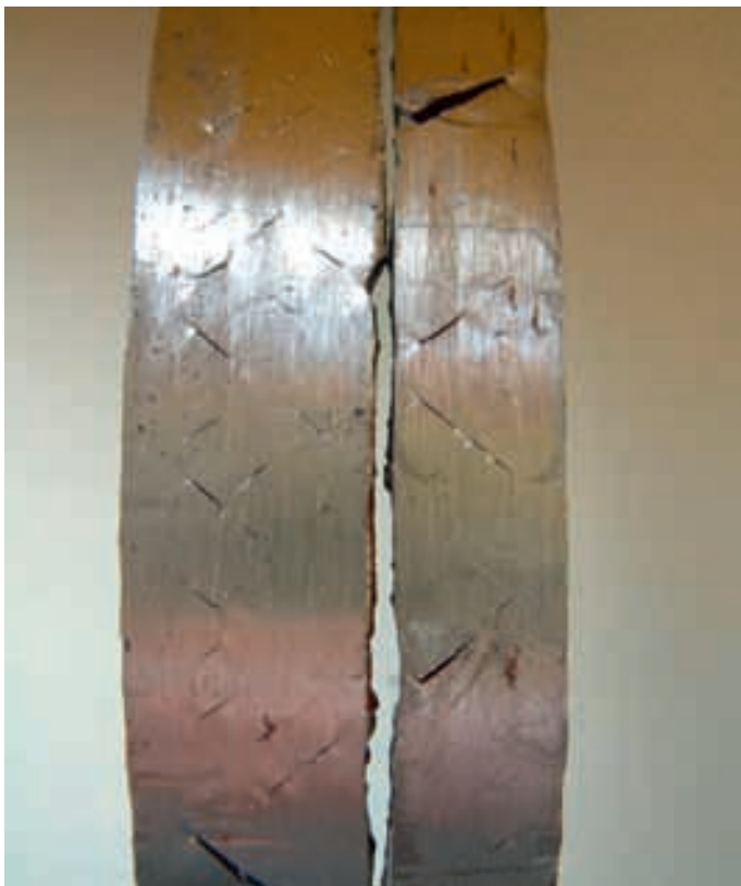
Figure 26: Bent specimens with widened cracks
