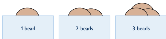
Figure 17: Seam structure when welding with different numbers of beads
